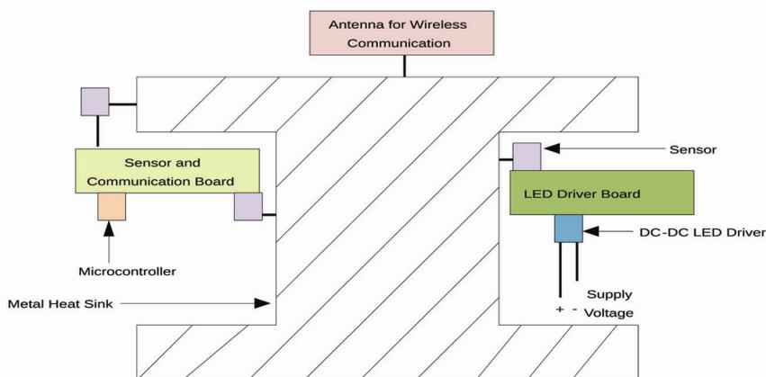
Figure 1. Visible light communication module.
