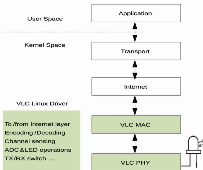
Figure 2. Communication stack of VLC in an embedded Linux operating system.
