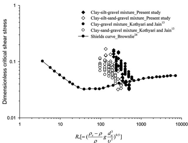
**Figure 1.** Variation of dimensionless critical shear stress with particle Reynolds number for cohesive sediment mixture and cohesionless sediment.
