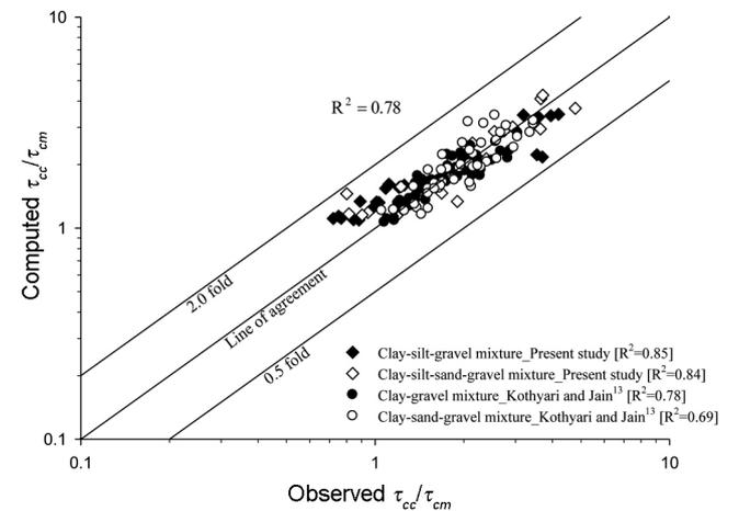
Figure 5. Comparison of observed and computed value of  $(\tau_{cc}/\tau_{cm})$  using eq. (7).
