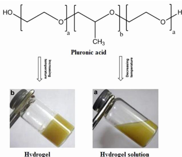
**Figure 6.** Response of pluronic acid (poloxamer)-based hydrogel to temperature.
