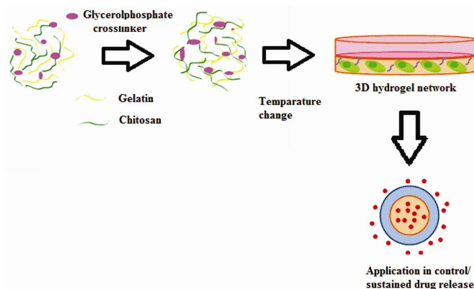
Figure 2. Schematic representation of chitosan-based thermosensitive hydrogels.
