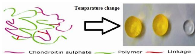
Figure 5. Chondroitin sulphate-based thermosensitive hydrogel.
