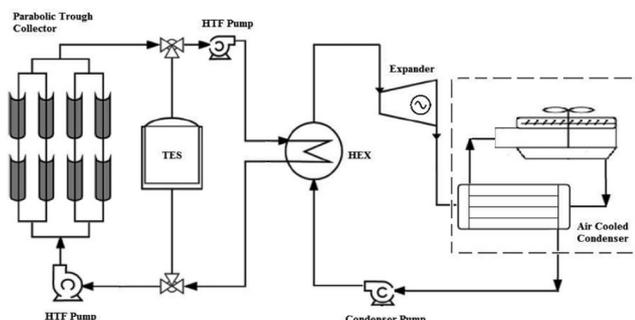
**Figure 1.** A schematic of a typical concentrated solar power plant with thermal storage system<sup>24</sup>.
