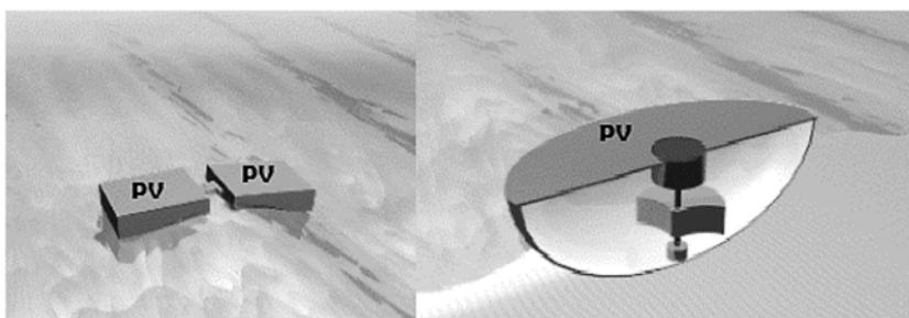
Figure 1. Wavevoltaic attenuator and wavevoltaic rotating mass devices.
