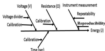
Figure 2. Cause and effect diagram (fish bone diagram) for depicting uncertainty components involved in energy measurement of defibrillator analyzer.
