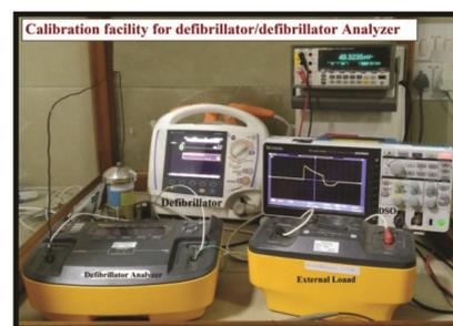
Figure 4. A set-up of calibration facility for defibrillator analyzer and defibrillator machine.
