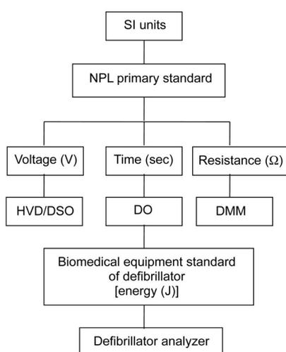
Figure 3. Flow chart of traceability chain of primary standard of defibrillator with traceable supporting equipment of high voltage divider (HVD), digital oscilloscope (DO) and digital multimeter (DMM).
