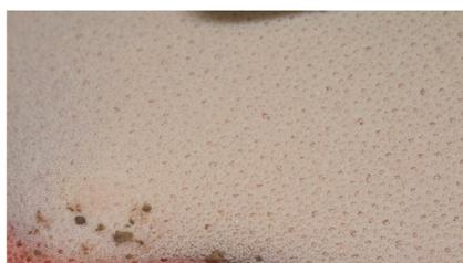
**Figure 2.** The pore surface on the underside of the specimen.
