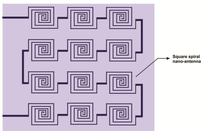
**Figure 4.** An array of square spiral nano-antennas.
