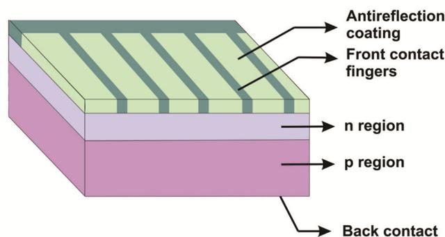
**Figure 3.** Basic structure of a p–n junction solar cell.
