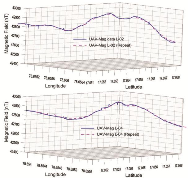
Figure 4. Repeatability of UAV magnetic data along lines 02 and 04.
