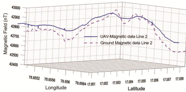
Figure 3. Ground and UAV magnetic data along Line 02.
