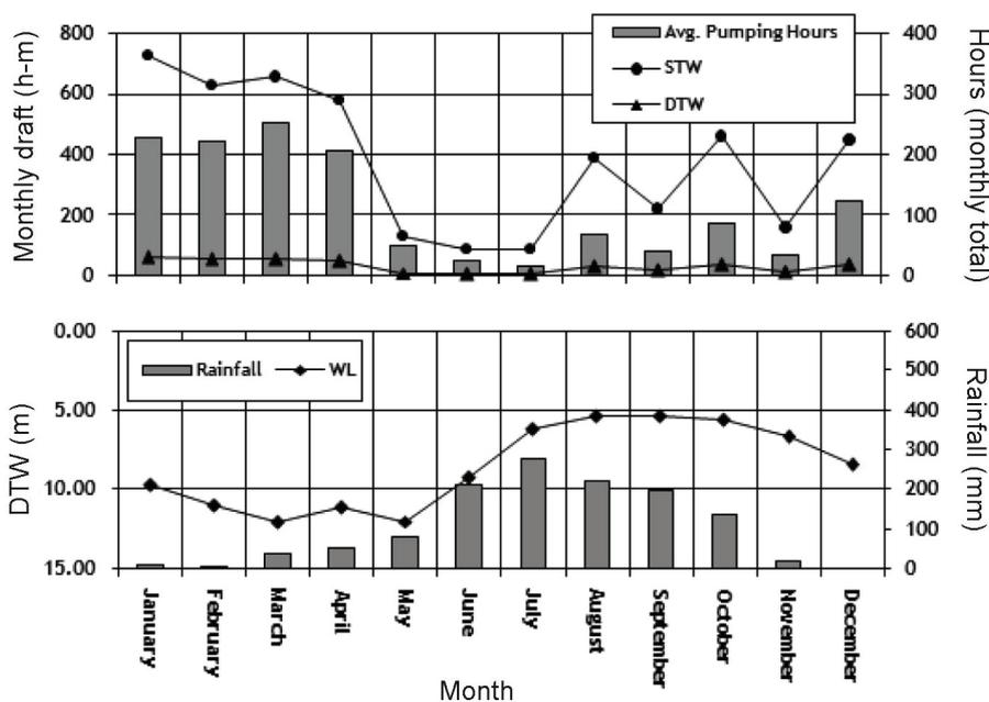
**Figure 3.** Variation in monthly draft of STW and DTWs against average monthly pumping hours, rainfall and depth-to-water level in Jangipara Block, West Bengal.
