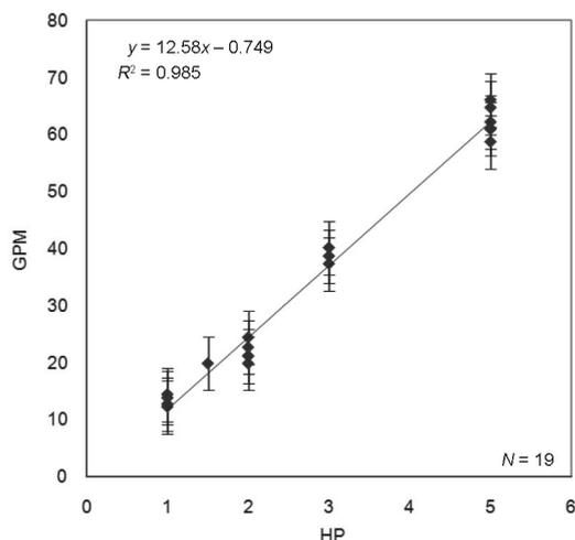
Figure 1. Measured discharge versus rated pump capacity.
