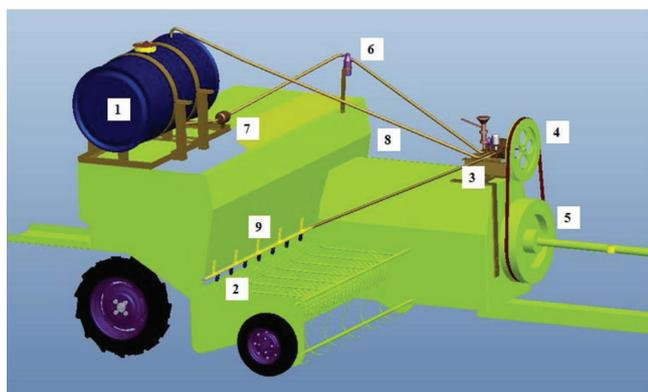
**Figure 1.** CAD view of the developed mechanized urea spraying system. (1) Urea solution tank; (2) flat fan nozzles; (3) HTP pump assembly; (4) belt and pulley; (5) fly wheel; (6) strainer; (7) cut-off valve; (8) pipe; (9) boom arm.
