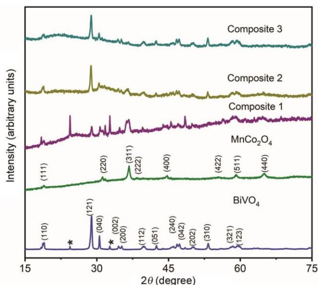
**Figure 1.** Powder XRD patterns of as-prepared  $\text{BiVO}_4$ ,  $\text{MnCo}_2\text{O}_4$  and their composites (\* indicates peaks from secondary tetragonal  $\text{BiVO}_4$  phase).
