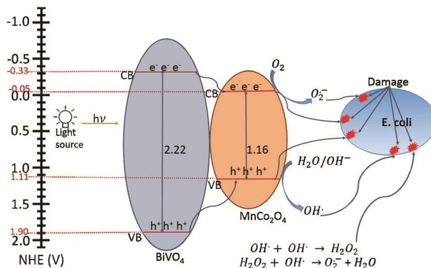
**Figure 6.** Visible light-induced charge carrier transport and proposed mechanism for the inactivation of *E. coli*<sup>27–32</sup>. NHE, Normal hydrogen electrode.
