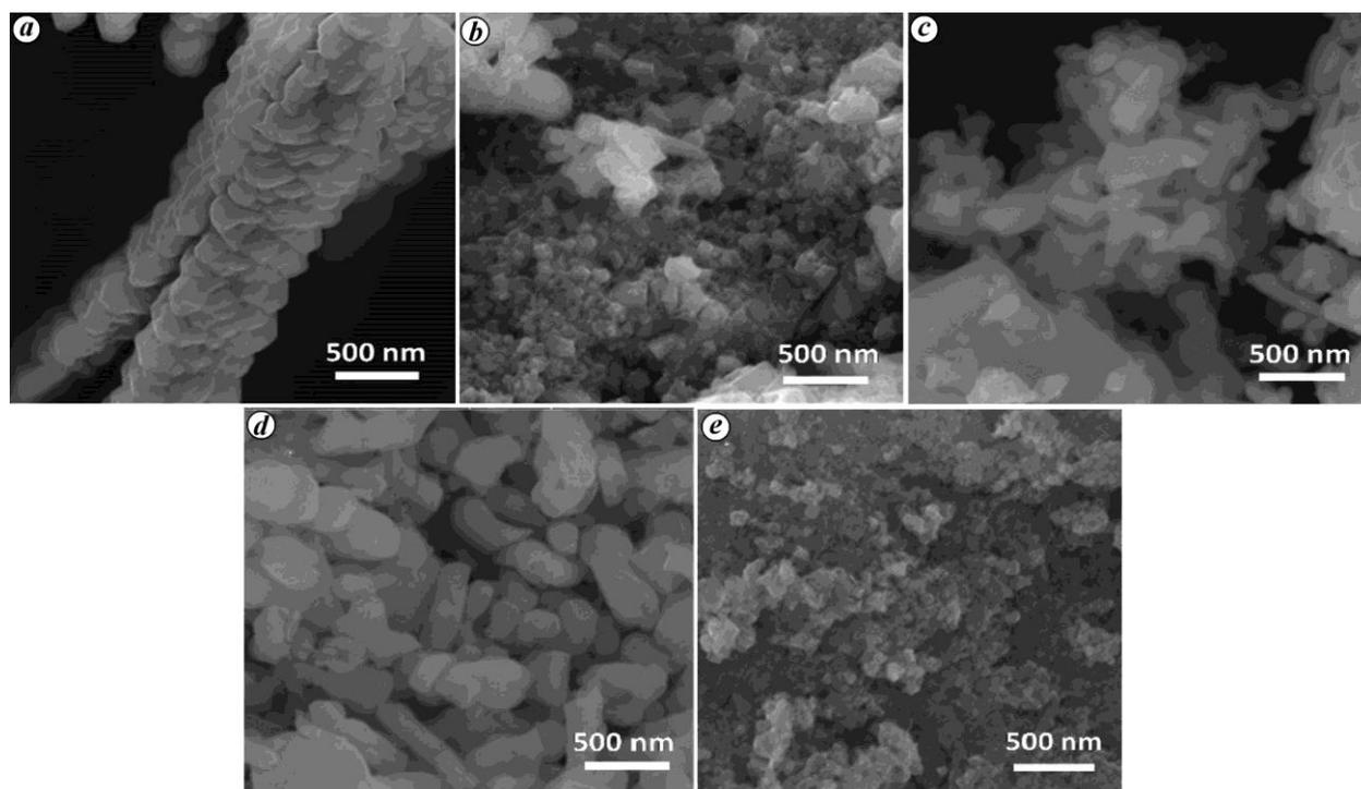
**Figure 3.** SEM images of as-prepared BiVO<sub>4</sub>, MnCo<sub>2</sub>O<sub>4</sub> and their composites. (a) BiVO<sub>4</sub>, (b) composite 1, (c) composite 2, (d) composite 3 and (e) MnCo<sub>2</sub>O<sub>4</sub>.
