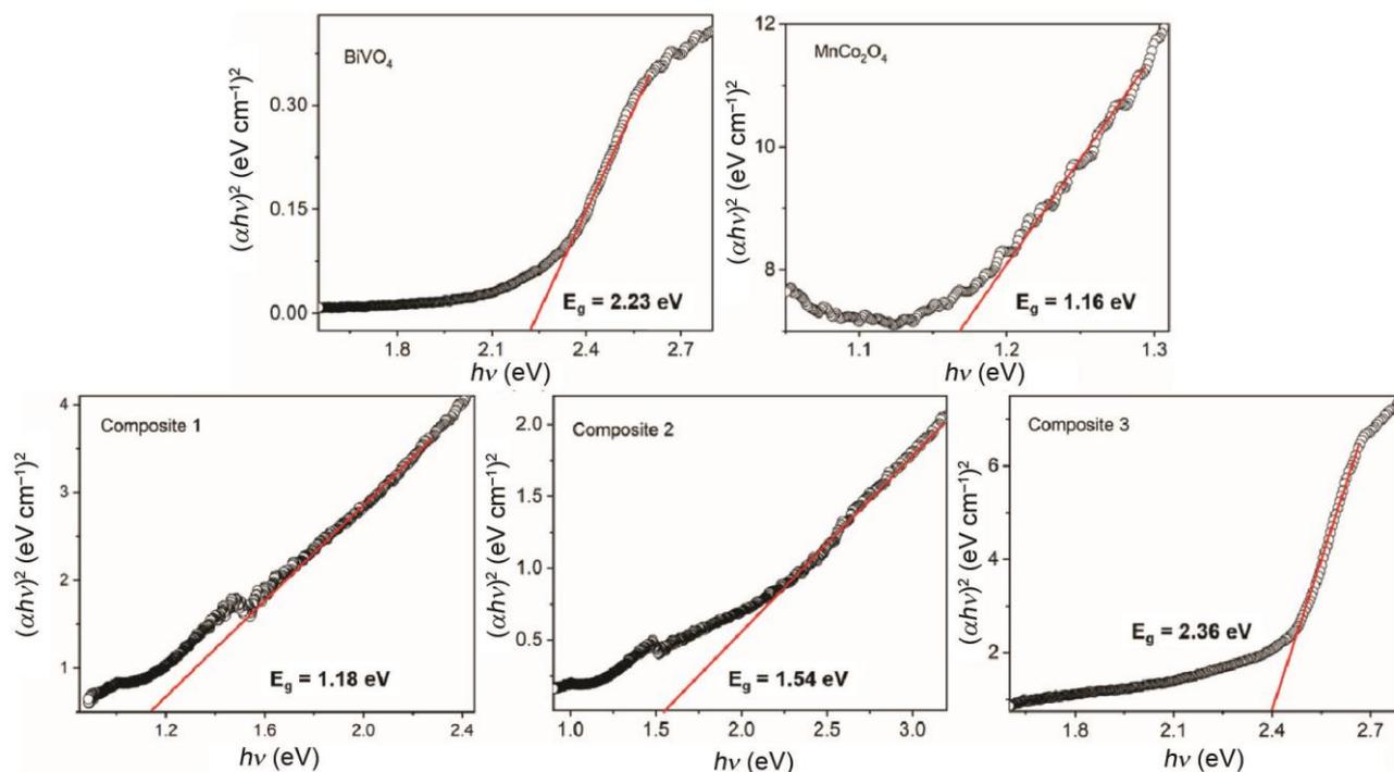
**Figure 2.** Tauc plots to determine band gaps of all the as-prepared compounds estimated using absorption data from diffuse reflectance spectra.
