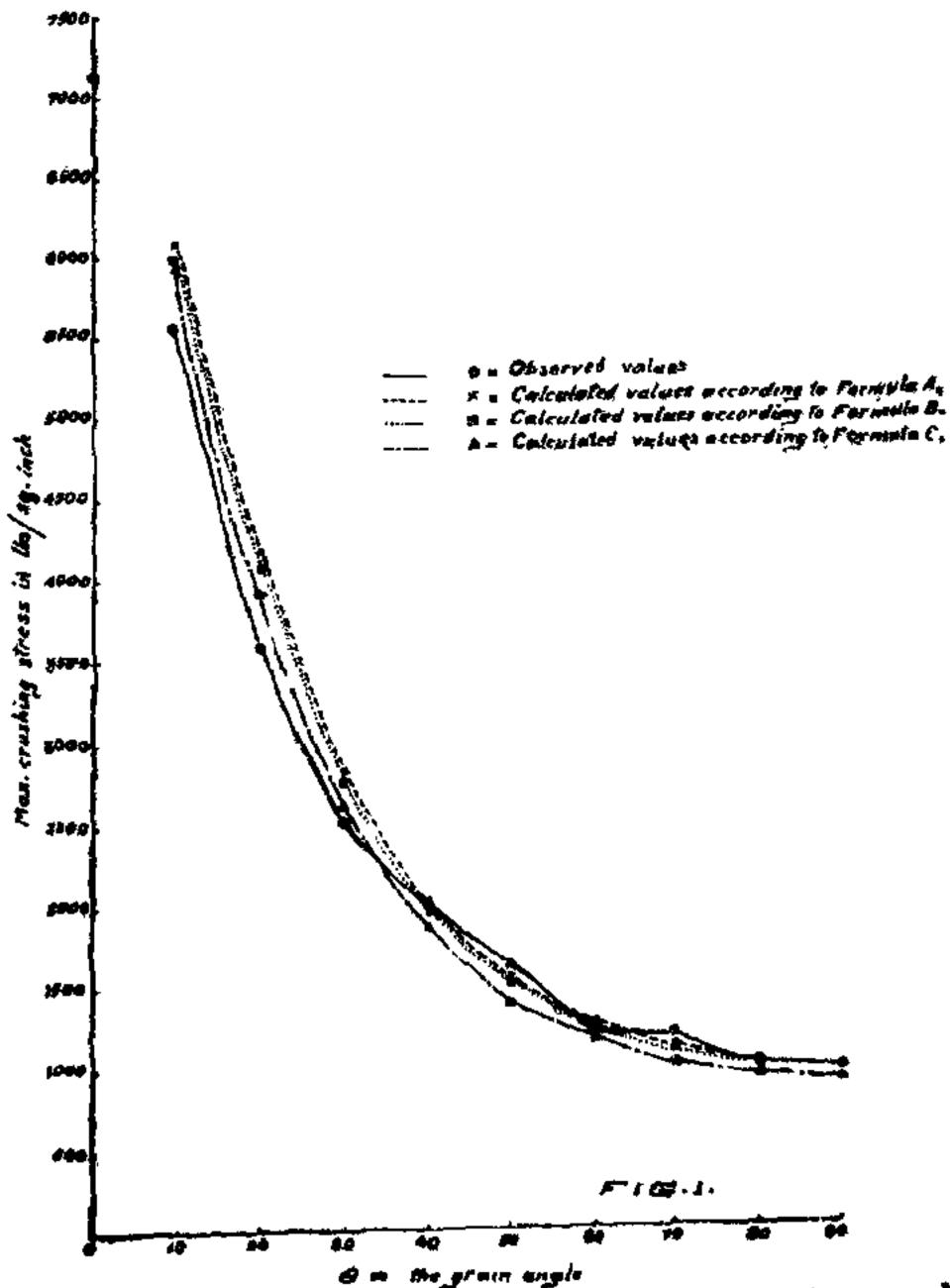
Theoretical.—In Figs. 1 and 2, the observed values and the calculated values according to the different formulæ are plotted against various angles of grain to the direction of force for maximum crushing stress and crushing
