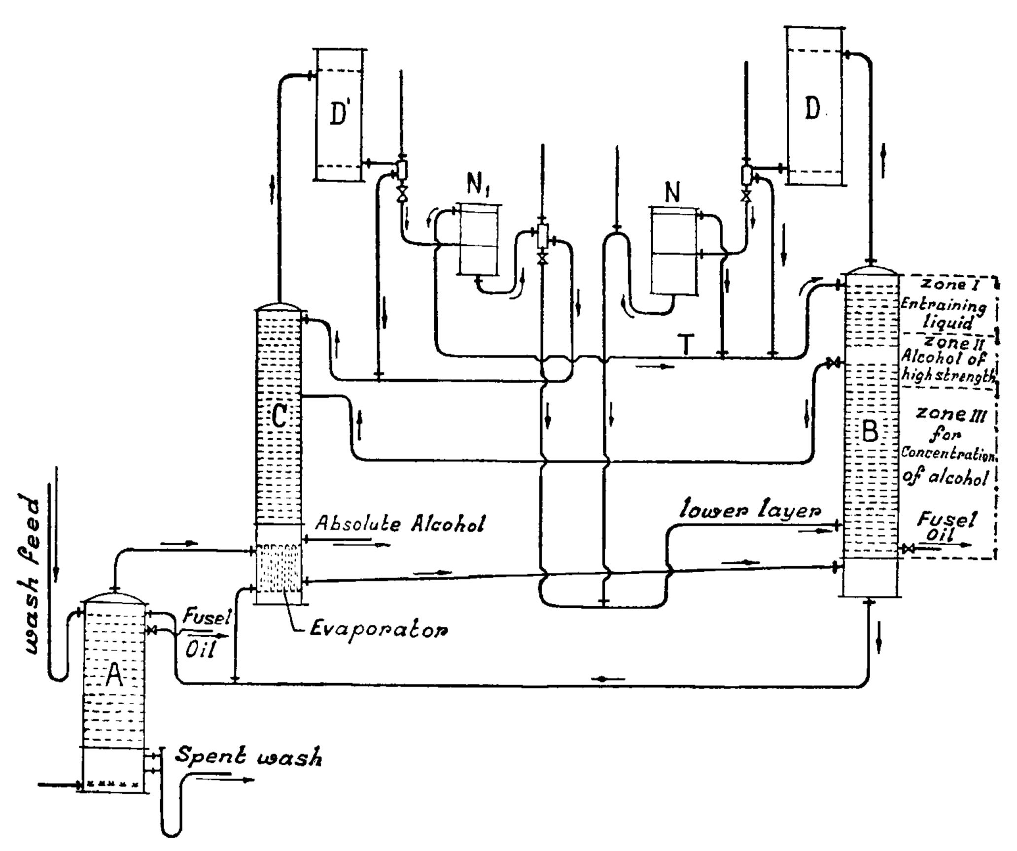
there is found a range of 4-5 plates containing alcohol of high strength (98.5-99 per cent.) mixed with a little of the entraining liquid. A suitable quantity of mixture is sent into the column C which is heated at the surface, and in which by continuous distillation it is possible to drive out completely the small quantities of water and entraining liquid present.
