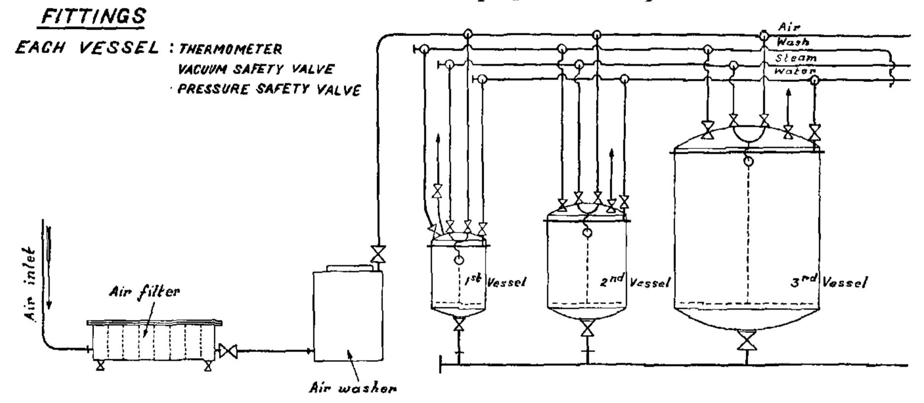
capacity of 22, 55 and 330 gallons. As each of the three basins must be sterilised, aerated, cooled and connected with each other, they are fitted with 4 sets of pipes. Each basin is fitted with a pipe to convey the sterilised air, and a coil to carry either steam for sterilisation or water for cooling.
