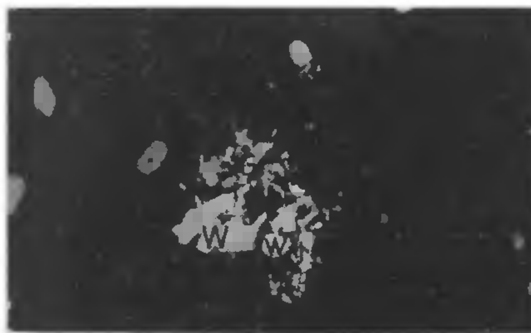
FIG. 2. Photomicrograph of basic rock showing fragmented clusters of ultrafine uraninite grains (grey) pyrrhotite (white, W), and ilmenite (isolated, scattered grains), \times 600 .
