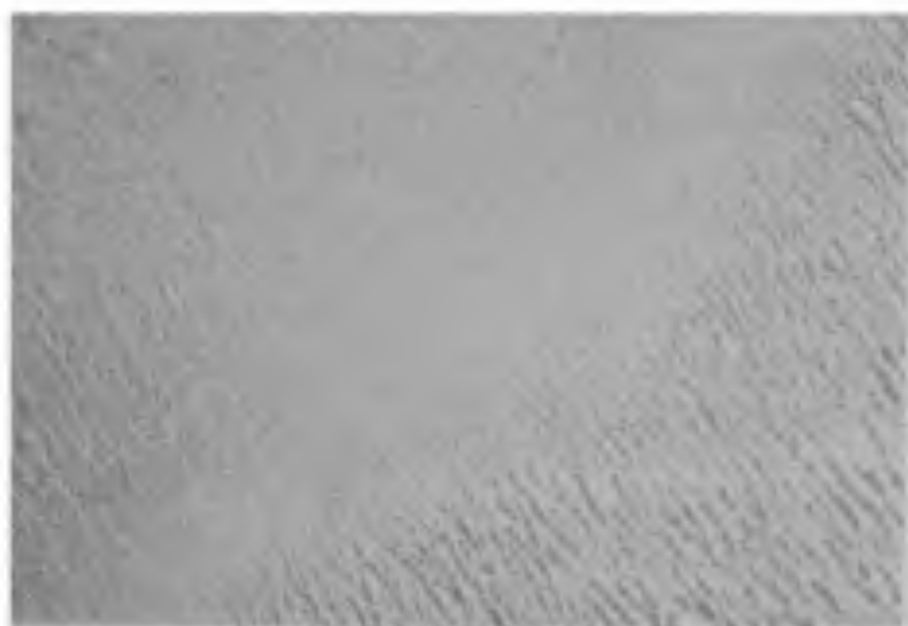
Figure 2. Ridge type of growth aligned in [110] direction when copper is deposited from acid copper sulphate bath in presence 5 \times 10^{-16} m/l of DTE at 2 mA/cm, \times 625 .
