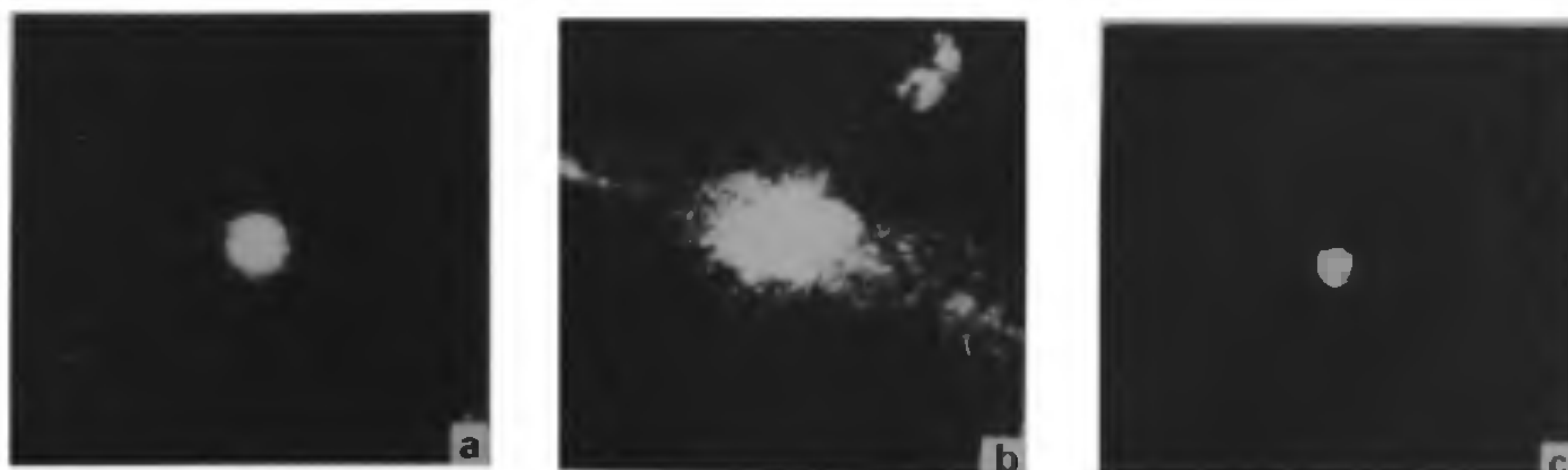
Figure 5a,c. Distortion correction properties of Phase Conjugate Beam. a. Phase conjugate beam; b. Probe beam after single passage through the phase distorter, and c. Conjugate beam after reverse passage through the phase distorter.
