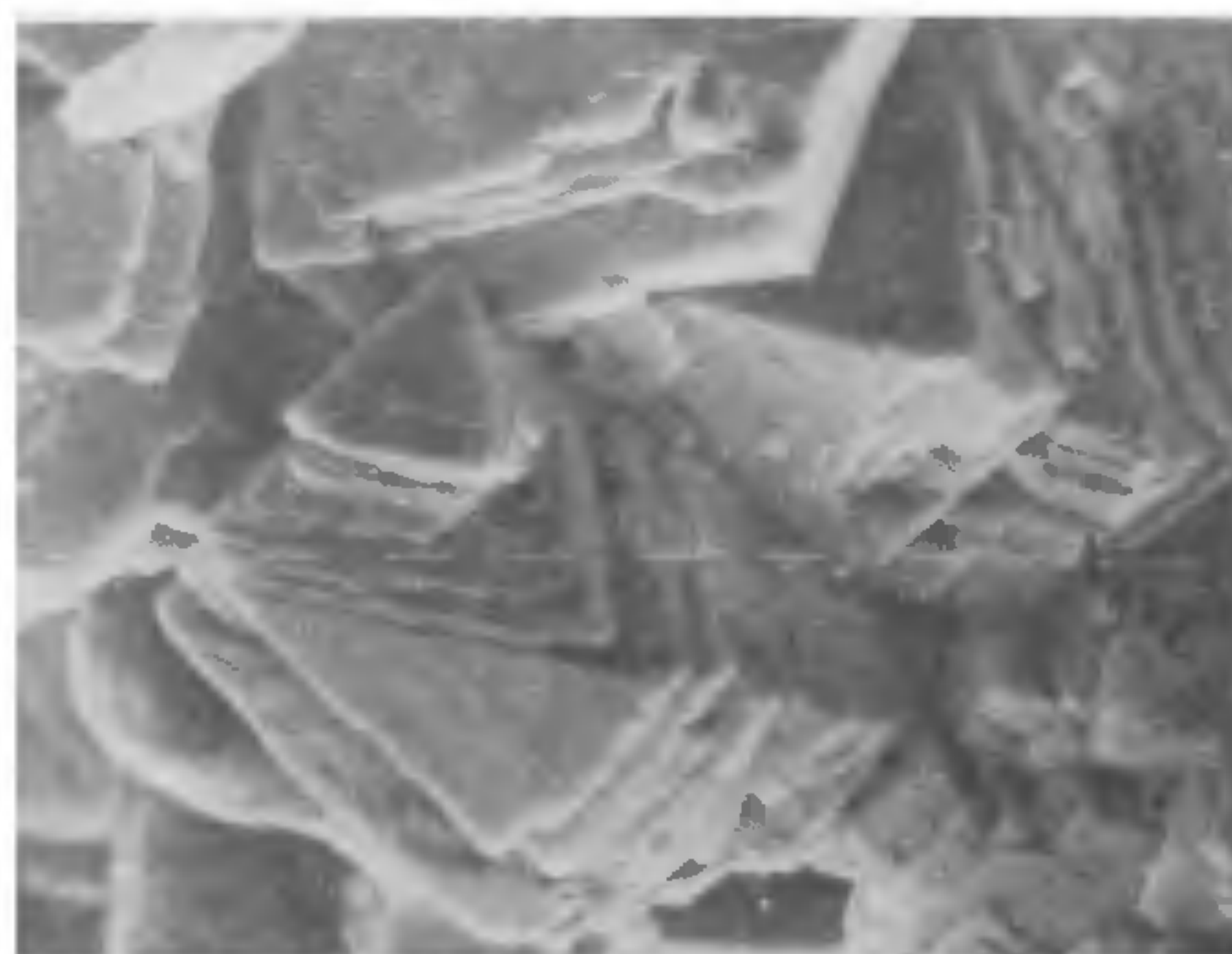
Figure 6. Scanning electron micrograph of C_{60} . The cubic morphology of the crystallites and the associated close packed (111) planes can be clearly seen.
