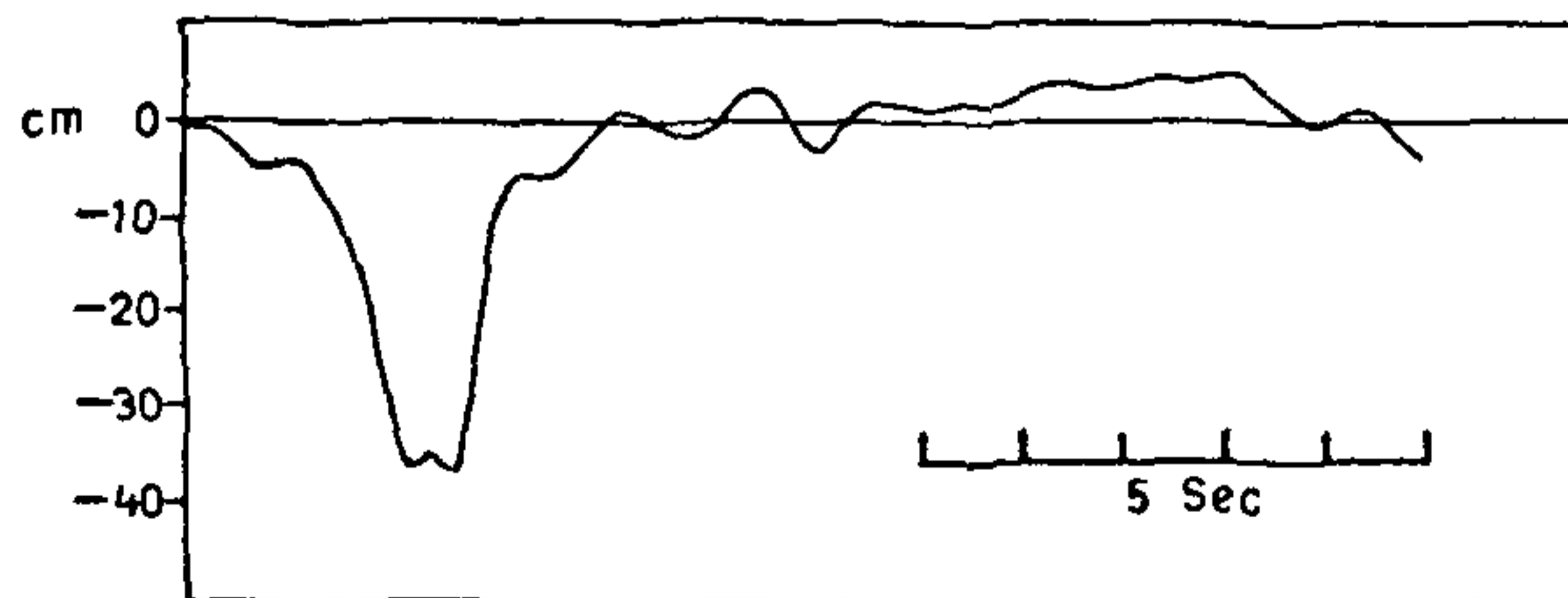
Figure 7. The displacement observed at 80 m from the San Andreas fault in the direction perpendicular to the fault trace during the 1966 Parkfield earthquake (after Aki, 1968).
