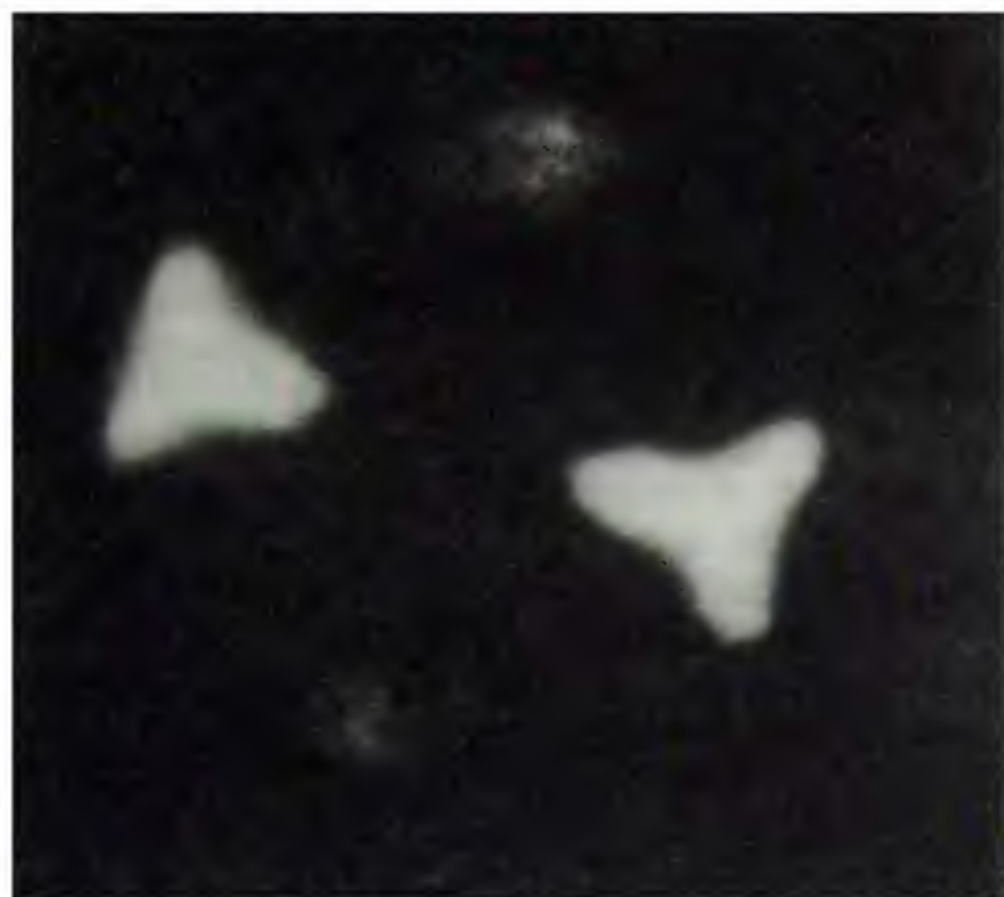
Figure 2. Field emission of nickel grown on tungsten field emitter. Highly stable emission is observed.
