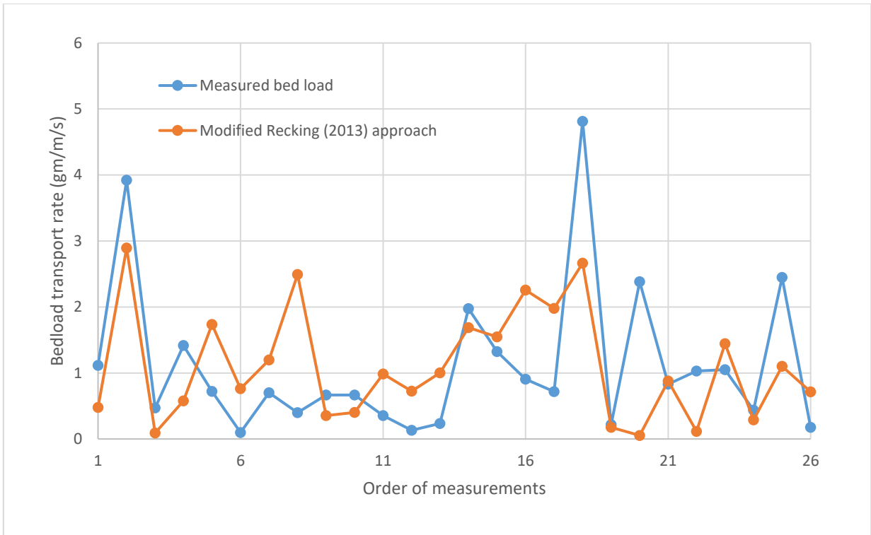
613 Fig. 7 Comparison of calibrated Recking (2013) relation and measured bedload rate
